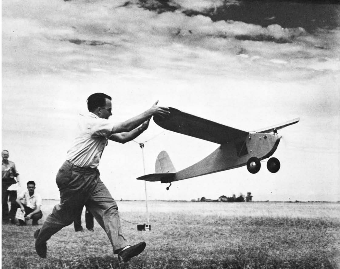
R/C has come a long way. The scene here is the 1937 Nationals with Bill Good, Walt's twin brother, assisting the "Big Guff" on its takeoff. The ship was basically a Free-Flight with escapement control of the rudder. The radio and batteries weighed nearly four pounds. This model was one of the first R/C birds to fly in the United States and is now resting in the Smithsonian Institute in Washington, D.C. A moment in our history that stirred the mind. Engine is a Brown.
